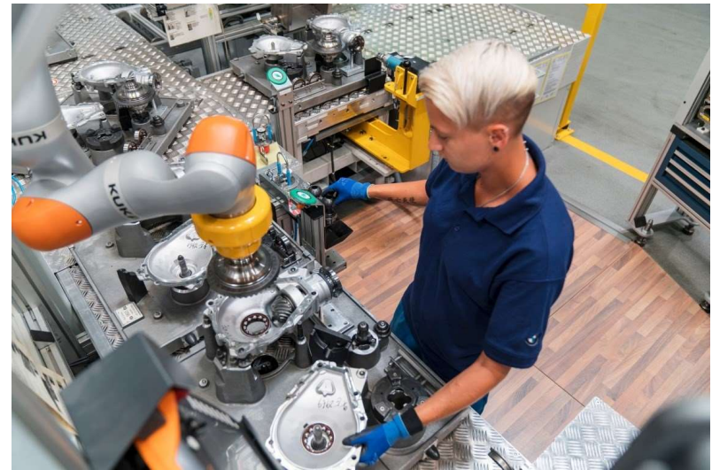
Allikas: BMW Group, Kuka, Human-robot collaboration in the axle drive assembly
