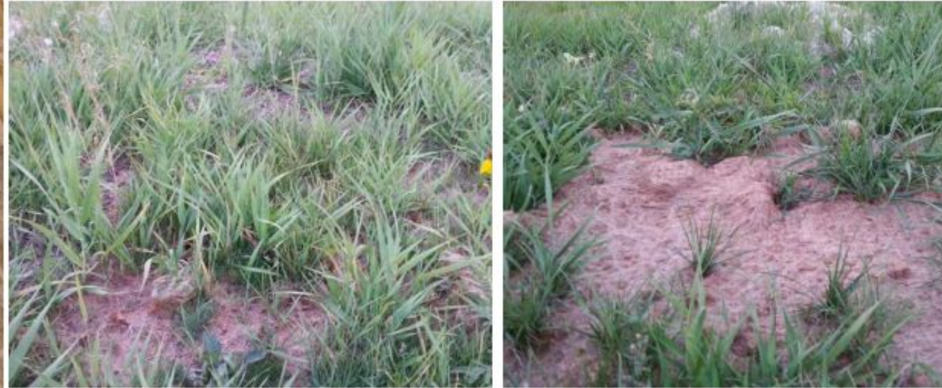
Figure 10: Seedlings are able to penetrate the 68 g/m 2 and 136 g/m 2 carded wool batting (left), but had difficulty penetrating the 203 g/m 2 and 271 g/m 2 carded wool batting (right).
