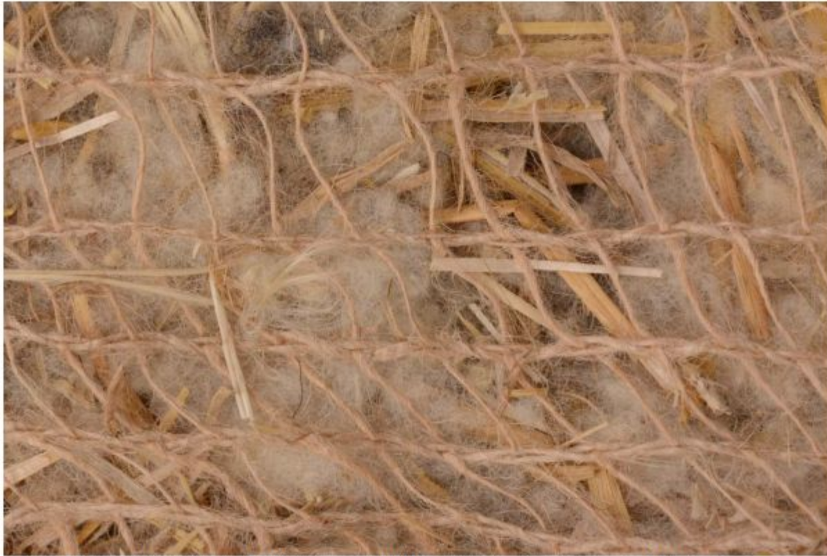
Figure 8: Close-up photograph of a 60 percent wool/40 percent straw erosion control blanket
